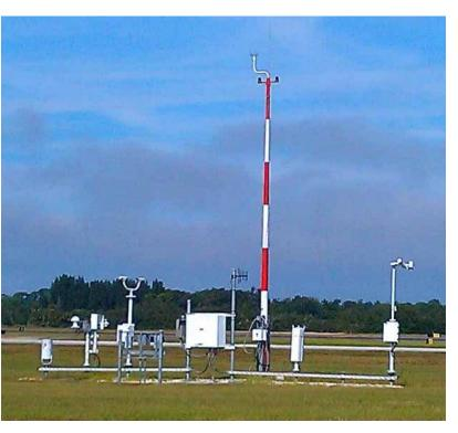
**CSG** (Combined Sensors Group) - **DCP** (Data Collection Package) and Sensors There are 571 FAA-owned ASOS in the.
