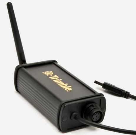
UX5 ground modem (2.4 GHz) straps to the tablet, connects to the tablet via its USB cable, and communicates with the aircraft via its RF antenna.
