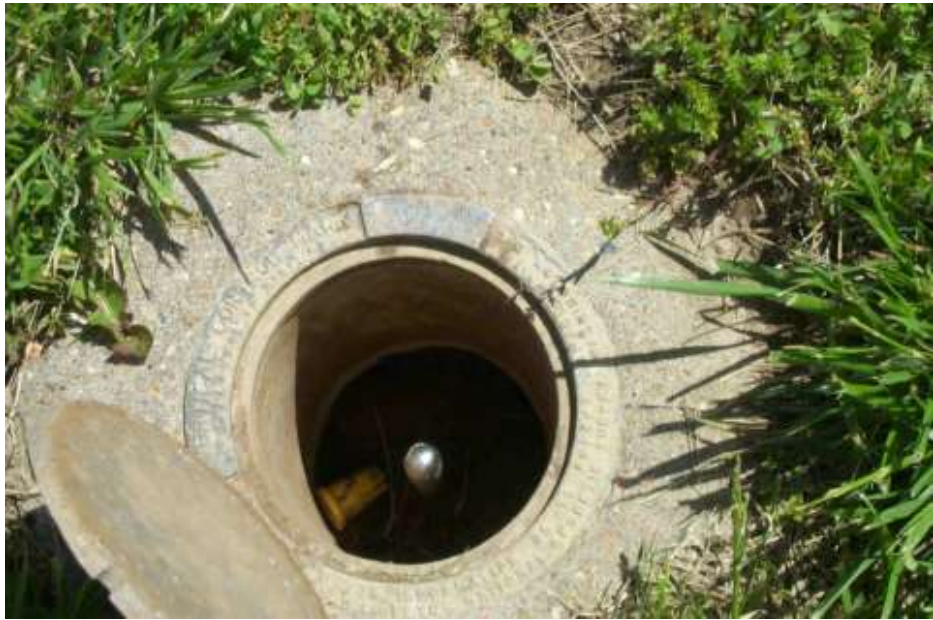
Stainless steel rod driven to refusal
